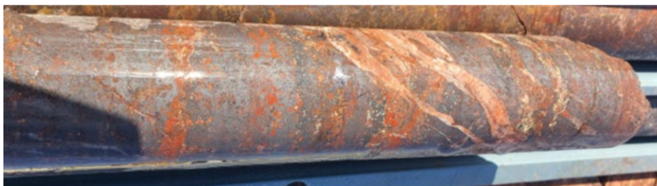
Figure 9 Haematite altered chalcite/bornite zone, 809.5m DD21EB0018W1. Veining is primarily baryte.
