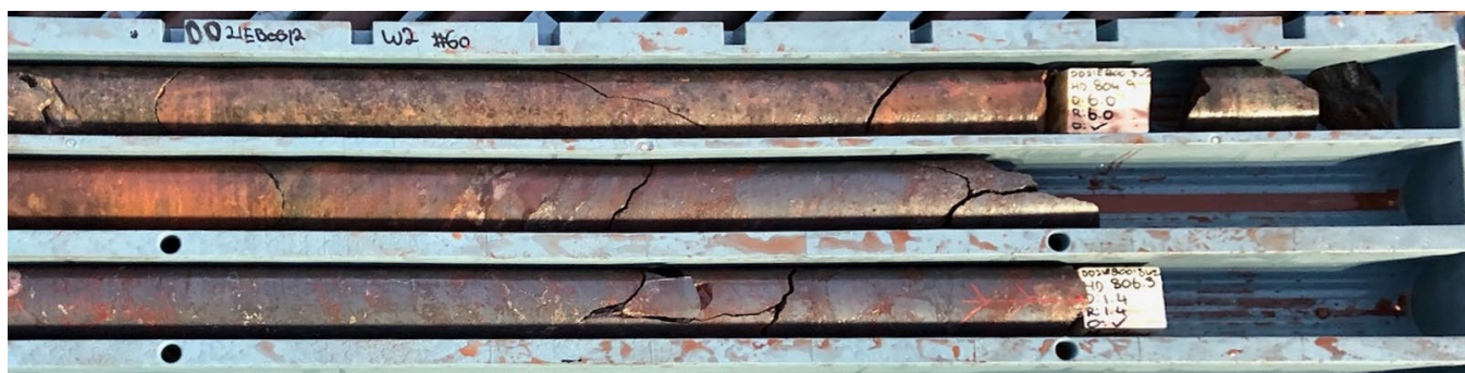
Figure 11 Transition from granite/haematised metasediments (pending identification) into steely haematite/chalcocite zone, DD21EB0018W2.
